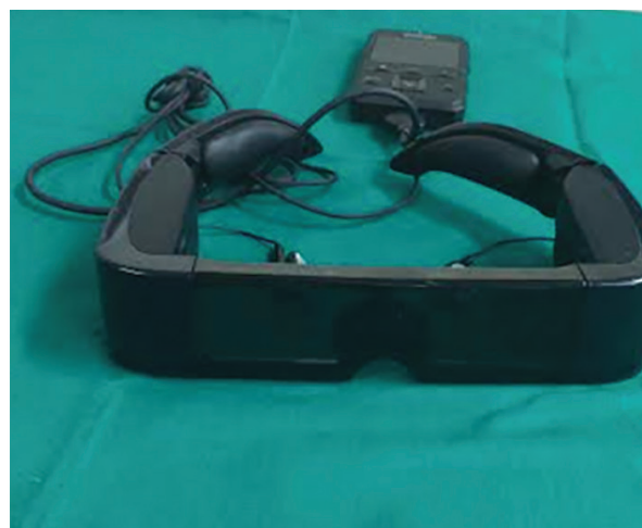
Fig. 2: Virtual reality smart glasses, detachable earphones, micro SDHC card
